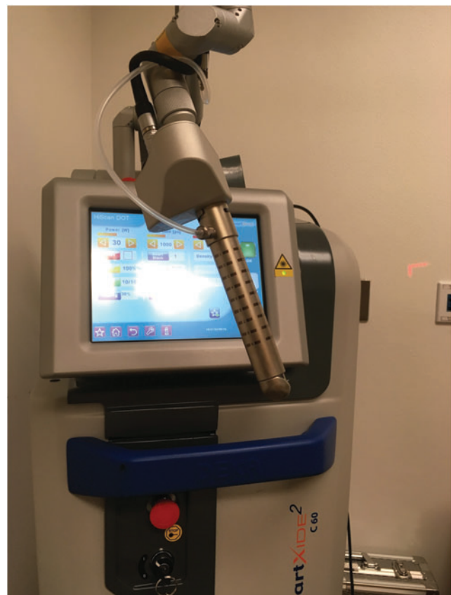
FIG. 1. The Monalisa Touch® SmartXide V2LR CO 2 laser with a vaginal probe attached to an articulated arm.
